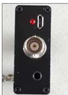
Left side with micro-USB for recharging, BNC connector and audio out
