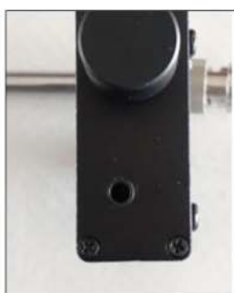
Right side with the encoder and the I/Q out, 3.5 mm stereo connector
